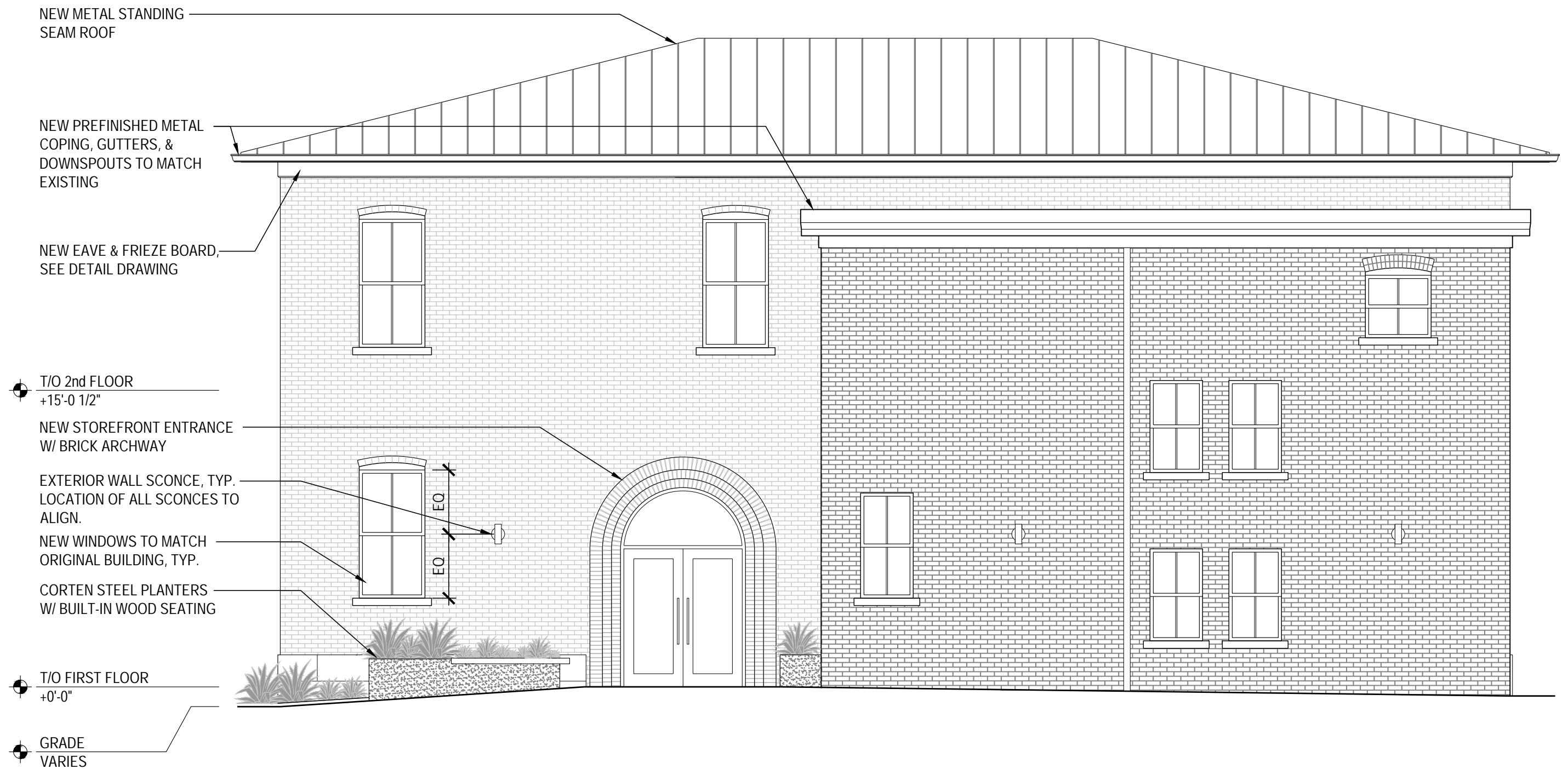
Proposed North Exterior Elevation
